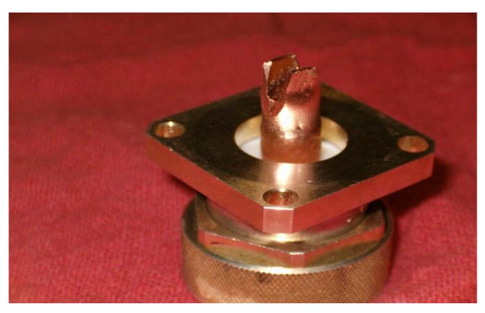
The Bullet is placed on the center connector and soldered, be sure to clean and smooth any excess solder. Wash with denatured alcohol and be sure it is dry before tinning the bullet and the shorting piece between the N connectors. Then assemble as outlined below.
