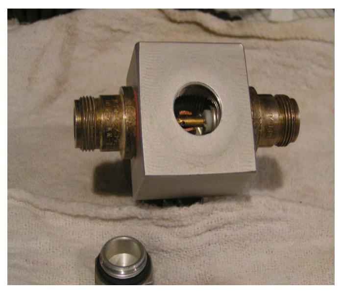
The grove that is filed into the end of the bullet is aligned so as to accept the solder pins from the two UG -680 connectors when assembled in the block.
