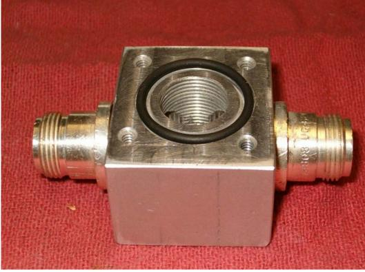
An "O" ring grove is machined under the DIN connector for weatherproofing and 4 holes are drilled and tapped to mount the 7/16 DIN connector. The block is drilled on 4 sides, 2 for mounting the UG-680 N connectors; one for mounting the 7/16 DIN connector; and on the opposite side for an access hole to allow for assembly.
