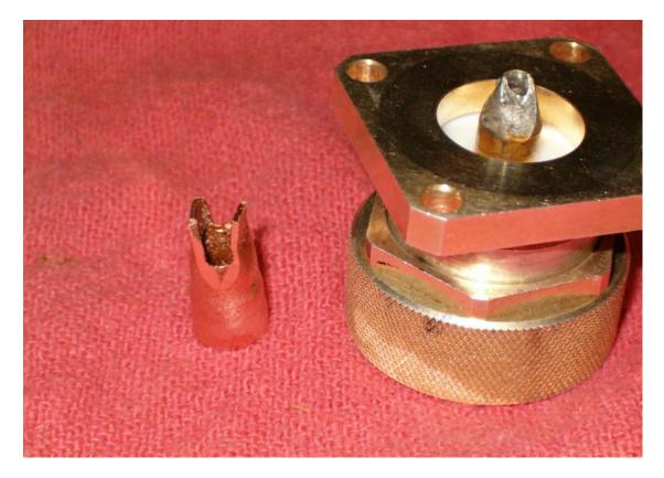
A copper "Bullet" is formed from tubing to make the short inner connection, I used a short piece of 5/16 copper tubing and hand worked the shape with a rounded end punch. I cut the slot with a hack saw and shaped it with a file.
