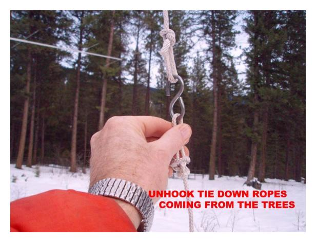
\_\_\_\_ Walk over toward the antenna where the tie-down rope is now slack. The tie down rope can now be unhooked from the line with the loop extending down from the cross boom. The tie-down rope with the hook secured to the end can be dropped to the ground.
