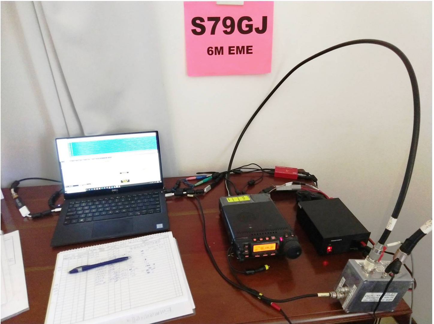
Note the clamp on ferrite filters on all the USB, power and audio leads connected to the computer. Ferrite filters are also used on all leads to and from power supplies, and the radio.
