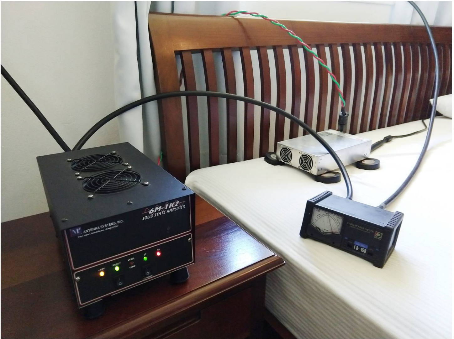
The rolls of plastic electrical tape under the Meanwell 50 VDC power supply were just to provide ventilation under the power supply, rather than having it site directly on the bedspread.
