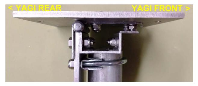
**STEP 9.** Use the two remaining bolts (part F) to bolt part E onto part D, placing a washer on each side of the channel leg. Tighten them while holding parts B and C at a small amount of adjust the position of the aluminum stop slightly- this is what prevents the yagi from pointing below zero degrees elevation.
