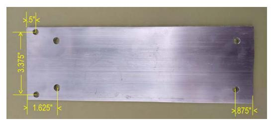
**STEP 2.** The mounting holes for the mast clamp U bolts should be located 1-5/8" in from the hinge (top) end of the plate and 7/8" in from the lower end of the plate.
