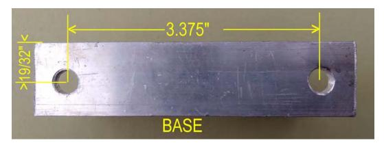
**STEP 4.** Drill two 5/16" diameter holes in the aluminum angle as shown.
