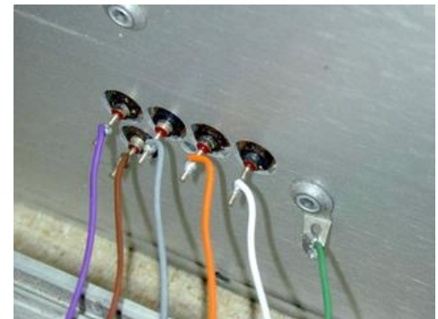
Front Panel LED Blink Code Wires
