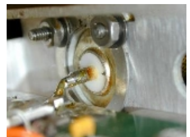
New RF output connector inside view. Note only 2 nuts used.
