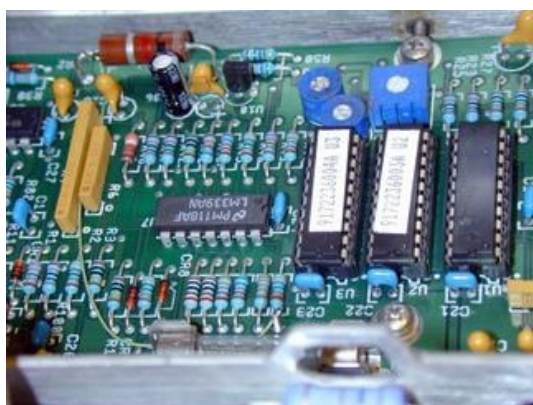
Control board, showing 3 PALs (center) and problem resistor R39 (upper left)
