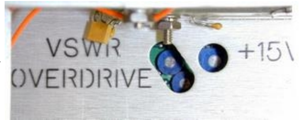
Control Board VSWR & Overdrive Adjustment Pots
