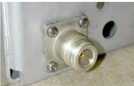
New RF output connector on chassis
