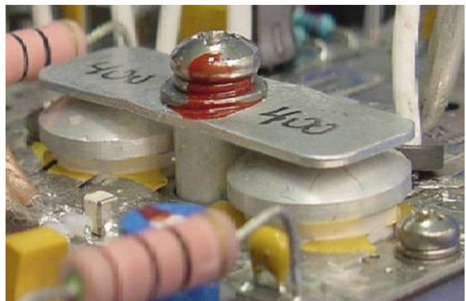
Device clamp to insure good thermal
