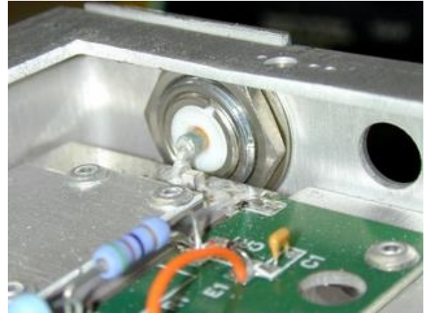
Original RF output conn., tuning cap and coupler
