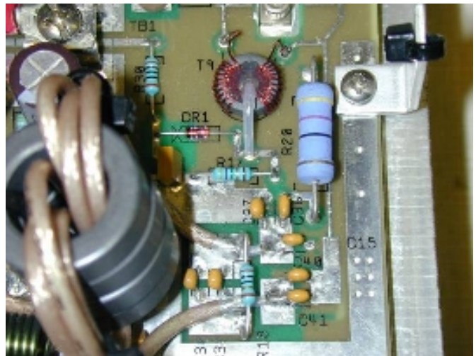
RF balance transformer and alarm
