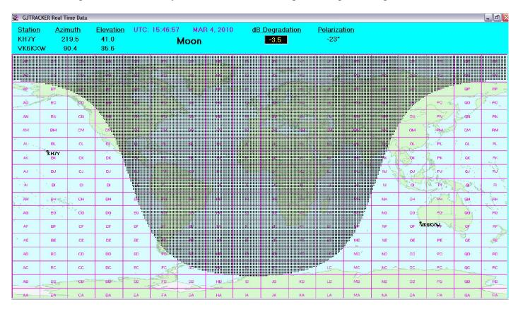
As you can see from the previous photo of the Real Time window, the data is displayed above a world map (courtesy of DX Atlas), upon which is displayed the approximate "terminator" for whatever object has been selected. As with the data at the top of the screen, the map is updated at the beginning of every minute. To view the entire world map, it is necessary to use a monitor capable of displaying at least 1280 by 768 pixels.
