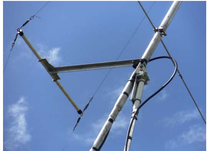
Closeup of hinged elevation mount with the yagi at high elevation
