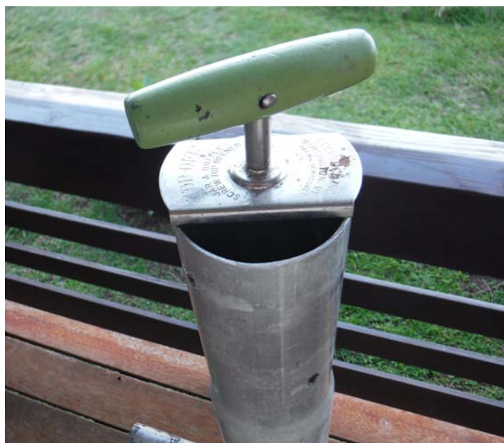
I brought a jar opener to re-round the larger tubing sections
