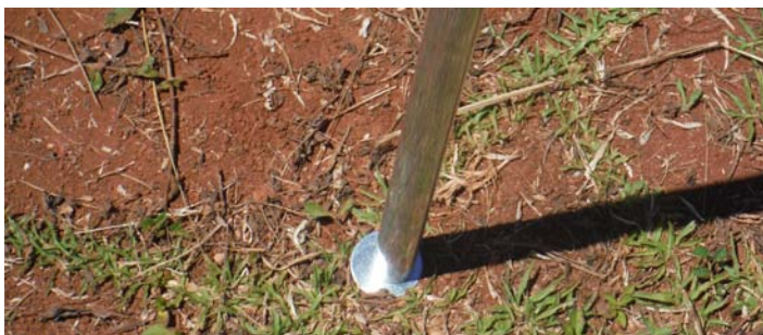
Upside down Prop mounted over a spike with a fender washer
