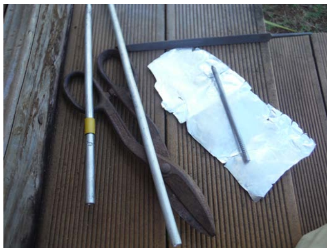
Fabricating the splice with a nail and pop can
