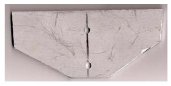
The spreader mounting piece is .75"  $\times$  1.5"  $\times$  1/8" thick angle aluminum 10.5" long. As can be seen in the scan below, a 5/8" deep saw kerf is made in the wide face of the angle aluminum, right at the angle. The ½" wide hose clamps will be inserted into those slots to secure the fiberglass spreader to the entire elevation mast.
