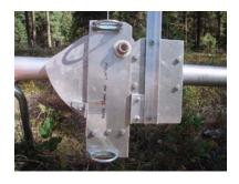
The mount was designed to be strong enough to withstand high winds, and provide safe, reliable service through multiple DXpeditions. The fabrication was done with hand tools using locally available materials. As depicted in this article, the mount will permit the 6M8GJ antenna to be elevated between 50 and 60 degrees.
