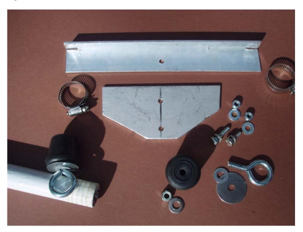
The 40" long piece of 1-1/8" diameter fiberglass spreader pole was (a remnant from the local University pole vaulting department of the Track and Field. These poles are used at the bars that are used at the top of the jumps. The "rubber tips" (rubber feet to fit over a walking cane) were purchased at the local hardware store and used as end caps for the fiberglass spreader. The spreader needs to be painted with three coats of marine fiberglass epoxy paint to protect it from UV degradation.
