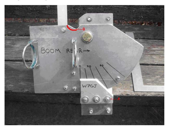
**NOTE** – By removing the bolt shown in the pressure plate at **A** and filing out the main plate as shown at **B**, the antenna can be raised to 65 degrees elevation.
