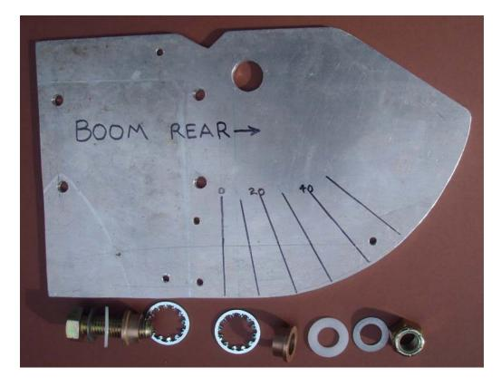
The pivoting boom plate is 9" high and the overall length from the flat front/left end to the tip on the rear is 14.75". The 1" diameter hole for the pivot bolt bearing flanges is located 7.5" from the flat front end, 1.5" down from the top edge. As you can see from the photo, the rear bottom of the plate is cut out with a saber saw
