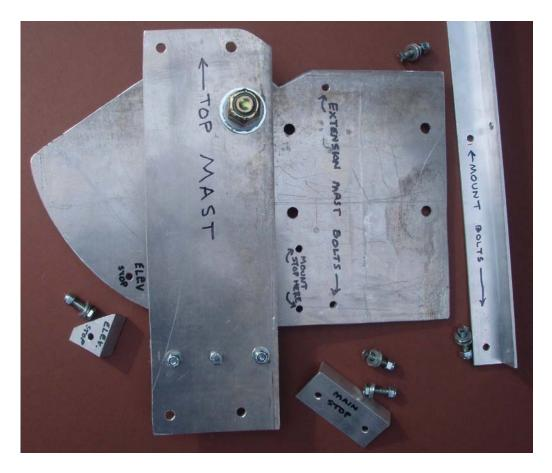
The above photo shows the mast plate mounted on the back side of the boom plate, along with the main stop, elevation stop, and extension mast. Hole locations for the extension mast, elevation stop and main stop can be scaled off the drawing or simply located after the mast plate is mounted together with the boom pivot plate.
