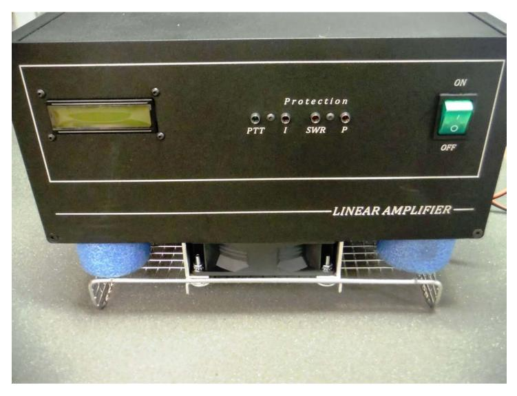
In August 2021, I purchased a 2kw solid state amp from EB104 for use during portable operations. The goal is to provide 1500w output on digital modes such as Q65, that are full duty cycle up to 50 seconds. In order to accomplish this, sufficient airflow must be assured.
