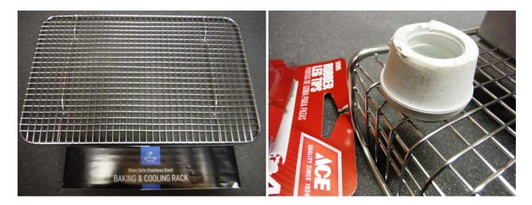
The two rails used to form the feet of the standard cooling rack were cut off, just leaving the bare rack. Each end then was bent down to provide sturdy support for the rack 1.75" above the desktop, while still permitting good airflow in from all sides. I don't have ready access to a metal brake to bend pieces such as the cooling rack, so I just placed the rack between two pieces of steel angle in a vise and bent it that way.
