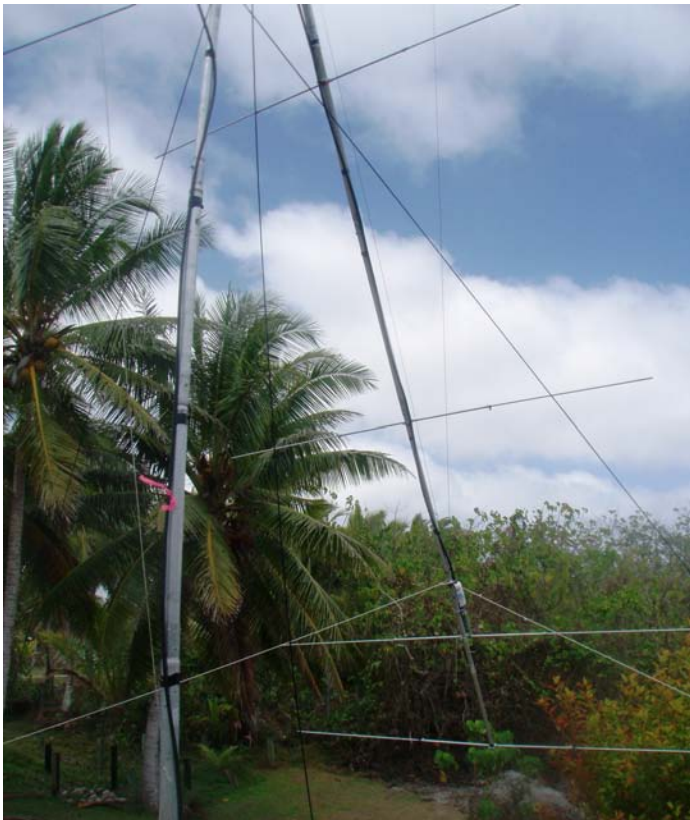
At maximum elevation, the guy ropes had to be interlaced between the elements as the azimuth was changed
