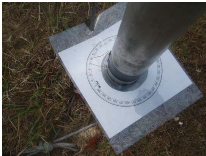
The W7GJ aiming circle and paper clip pointer installed
