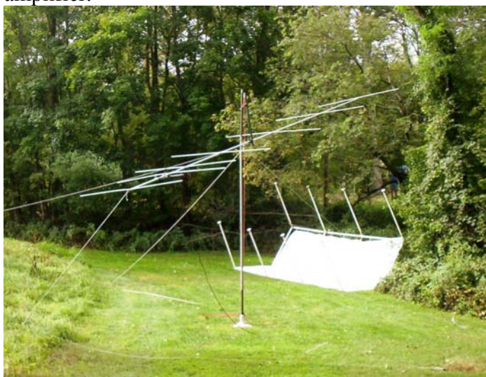
W1JJ's makeshift EME setup of an M 2 6M7JHV, manually elevated to 12° and pointed at the moon, with 700 watts
