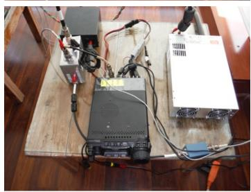
I always bring along a pair of 4' long LMR600 jumpers and a pair of LMR400 jumpers in addition to some short RG58 cables to connect all the equipment. I also had an extra 25' length of LMR600 coax that I did not need to add to the feedline this trip.
