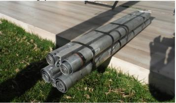
The horizontal fiberglass cross piece for the antenna boom guy lines, along with the mast from the elevation mount, the mast prop, the falling derrick and all the aluminum tubing from both the antenna and mast are all magically telescoped into a compact package no longer than 44".
