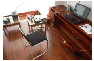
Note the liberal use of ferrite filters on all the leads coming out of the computer and any piece
