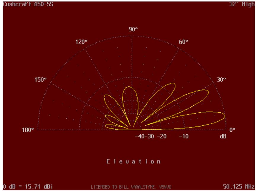
Figure 6: Stock A50-5S Elevation Plot
