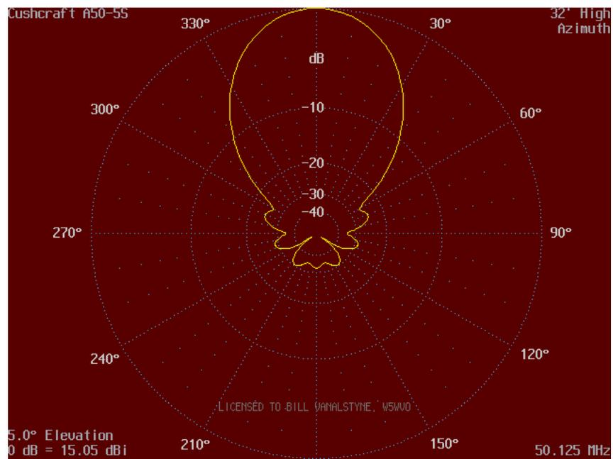
Figure 5: Modified A50-5S Azimuth Plot
