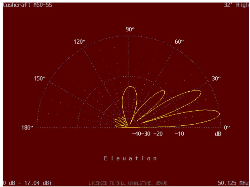
Figure 7: Modified A50-5S Elevation Plot
