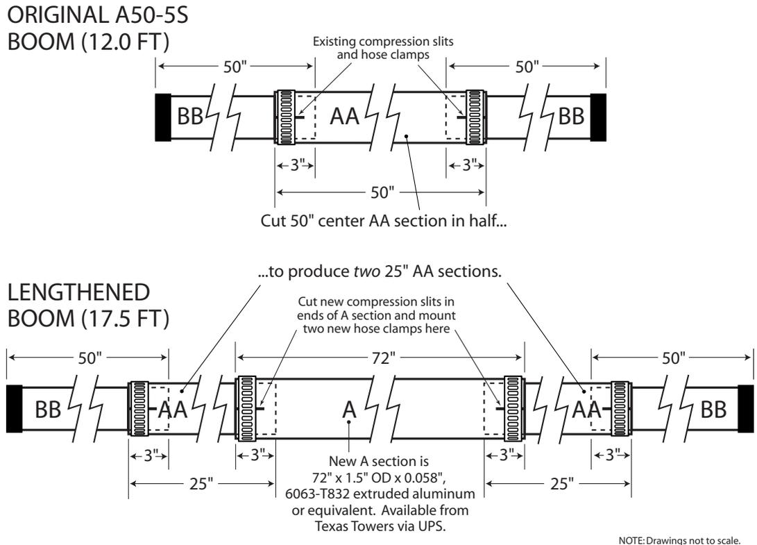
Figure 1: Original and Lengthened Boom Assembly
