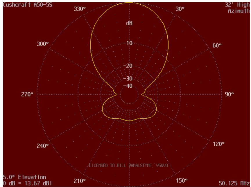
Figure 4: Stock A50-5S Azimuth Plot
