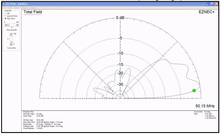
Antenna at 25° Elevation: Main Lobe at 23° elevation and 15.21 dBi (0.95 dB ground gain)
