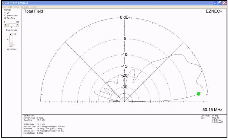
Antenna at 30° Elevation: Main Lobe at 22° elevation and 15.02 dBi (0.76 dB ground gain)
