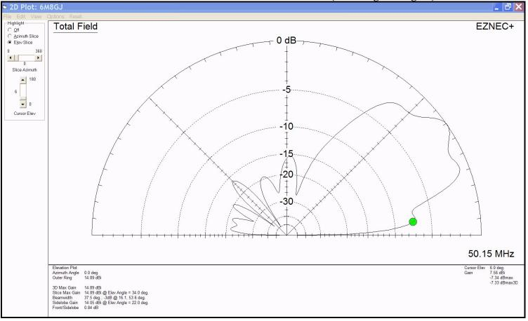
Antenna at 45° Elevation: Main Lobe at 46° elevation and 14.47 dBi (.21 dB ground gain)
