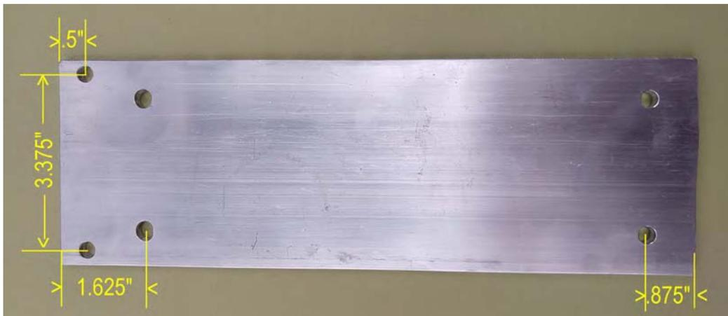
**STEP 2.** The mounting holes for the mast clamp U bolts should be located 1-5/8" in from the hinge (top) end of the plate and 7/8" in from the lower end of the plate.
